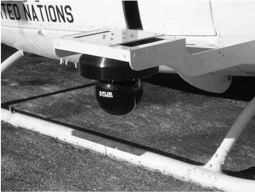
Figure 7.4 The pod containing the FLIR camera, attached to a Chilean helicopter in MINUSTAH.
